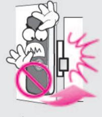
Please do not close the door with the deadbolt in the locked position. It may damage the product or cause a malfunction.
