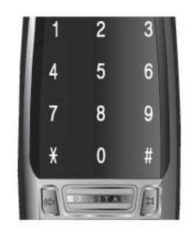
This model has touch type numeric pad. Numeric pad is turned on when you press start button or mute button.
