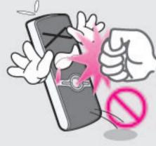
Do not force to pull the front cover. It may damage the product or cause a malfunction.
