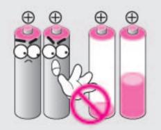
Please do not mix old with new batteries or use different types. Always use new alkaline batteries. Please make sure the batteries are inserted correctly (+/-) as indicated in the battery compartment. Otherwise, it may cause a leaks or explosions.
