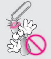
Do not allow the battery electrodes to make contact with metals such as keys, as the battery may overheat, causing explosion or severe damage.
